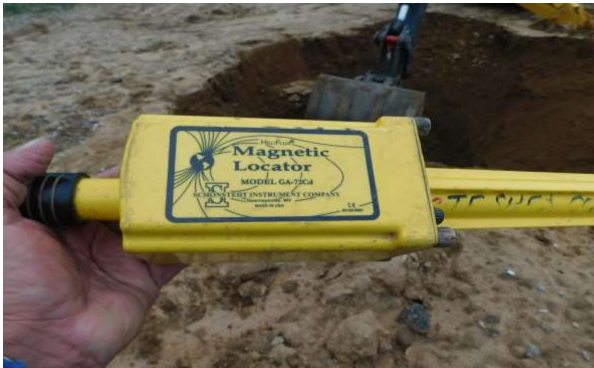
5. Looking at hand-held magnetic locator instrument used to locate well casing and direct excavation.
