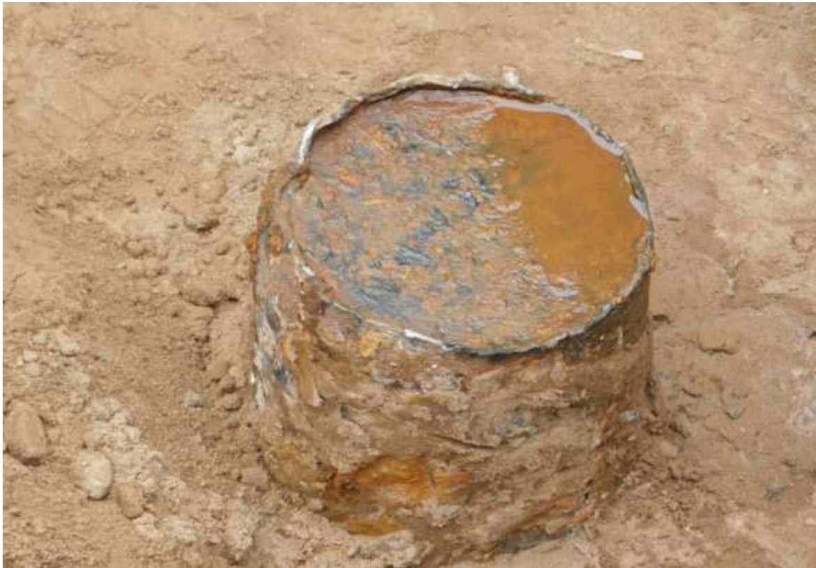
12. Close-up look at top of well casing in excavation pit after FID leak test and bubble test.
