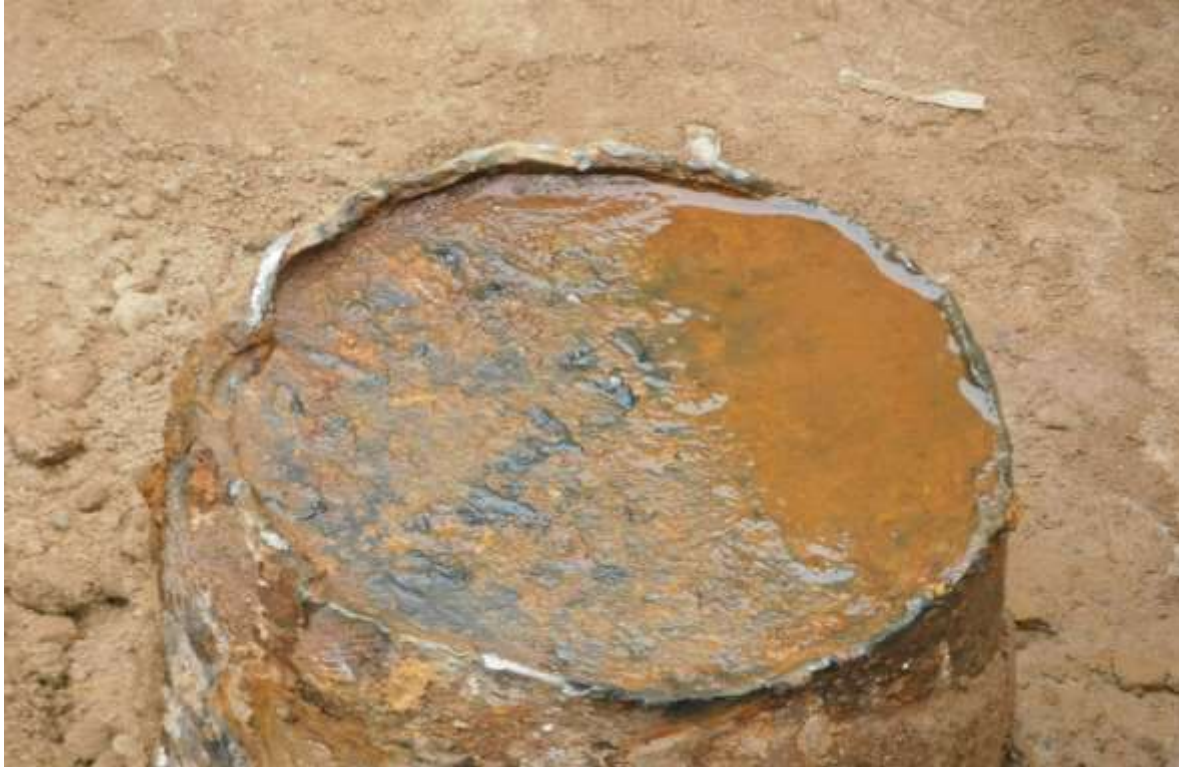
13. Close-up look at top of well casing in excavation pit after FID leak test and bubble test.
