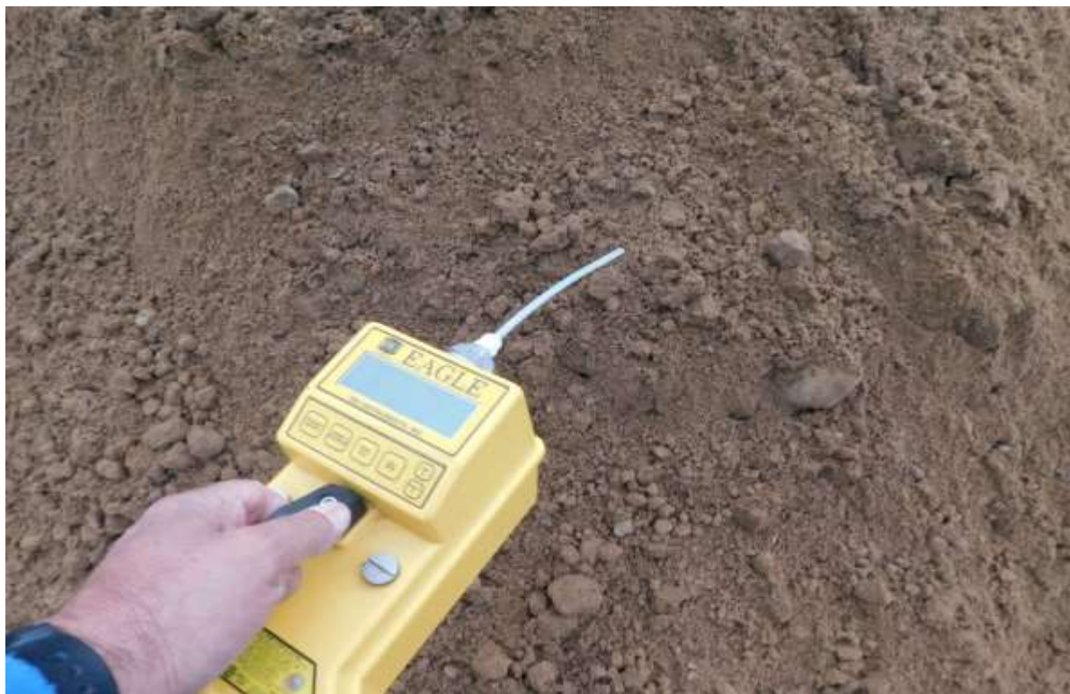
4. Looking down at soil monitoring procedure for excavated/stockpiled soil.
